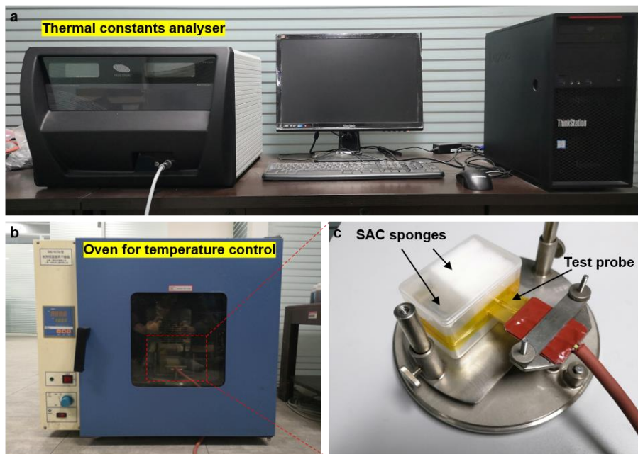
Supplementary Figure 27. Optical image of the thermal conductivity determination system. a Optical image of the thermal constants analyser, b optical image of the oven for temperature control, and c optical image of the test probe and SAC sponge samples.
