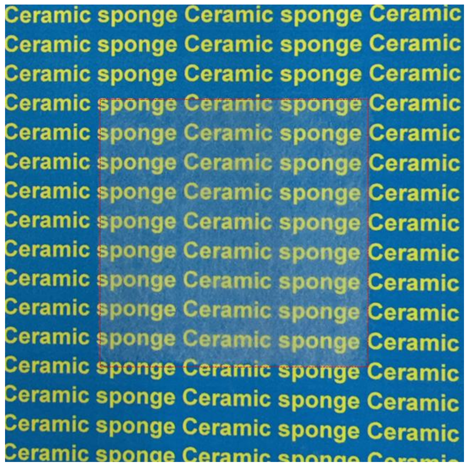
Supplementary Figure 16. Photograph of a single microfiber layer to show its transparency.
