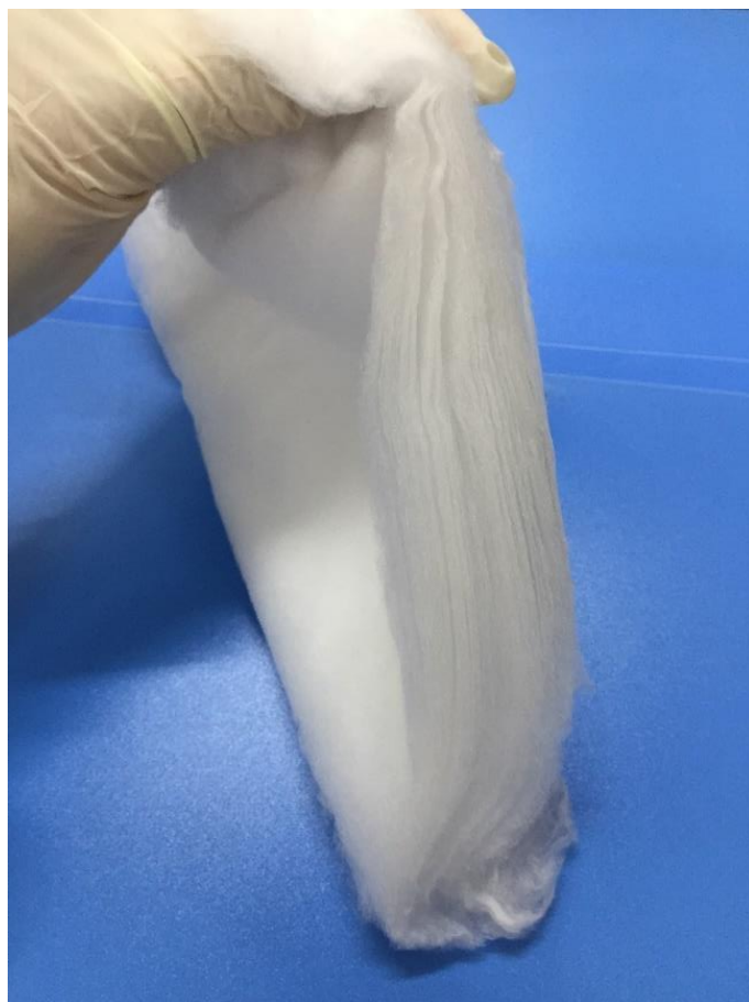
Supplementary Figure 7. Photograph showing the lamellar structure of the prepared PSAC sponge.
