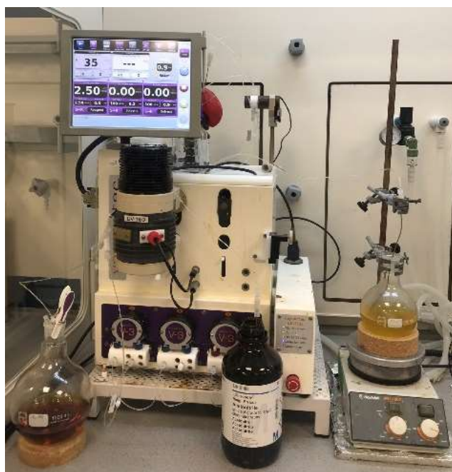
Figure S4: Scale-up experiment in continuous flow performed in a Vapourtec photoreactor
