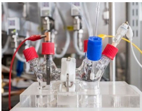
Supplementary Figure 1. Image of the three-electrode H-type electrochemical cell employed for electrolysis
