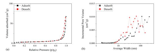
Figure S4. (a) N<sub>2</sub> adsorption-desorption curve and (b) BJH pore size distribution for M-phase.
