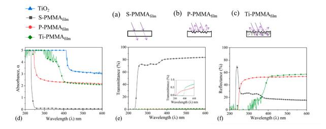
**Figure S1.** Schematic sketch of light interaction in the (**a**) S-polymethyl methacrylate (PMMA)<sub>film</sub>, (**b**) P-PMMA<sub>film</sub>, and (**c**) Ti-PMMA<sub>film</sub>. Optical properties characterized using UV-vis (**d**) absorbance (**e**) transmittance and (**f**) reflectance.
