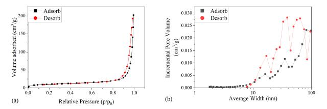
**Figure S2.** (a) N<sub>2</sub> adsorption-desorption curve and (b) Barrett-Joyner-Halenda (BJH) pore size distribution for D<sub>5</sub>.
