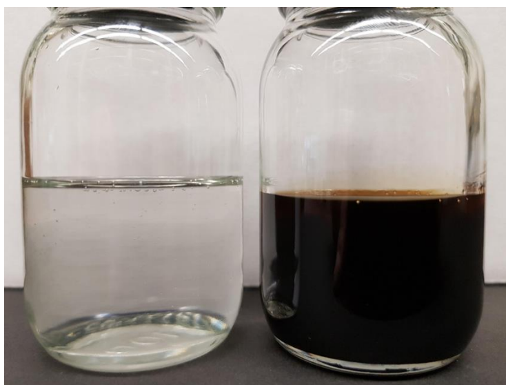
Figure 1S. Glycolysis product obtained from flexible PU foam waste and diethylene glycol at 1:1 (w/w) ratio, in autoclave (image at right), compared to the virgin polyol (image at left)
