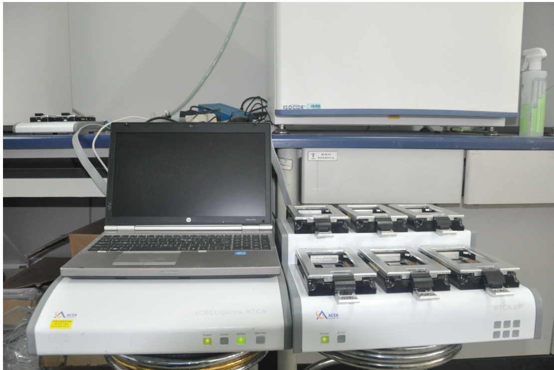
Supplement Figure 1. An image of the xCELLigenceRTCA MP system (ACEA Biosciences, Inc. USA) was used for this study. This instrument can monitor six 96 well plates simultaneously yet each plate is controlled independently from the other plates. The instrument is placed inside the tissue culture incubator. The cell growth and monolayer formation were monitored and controlled by the control unit and computer outside of the incubator.
