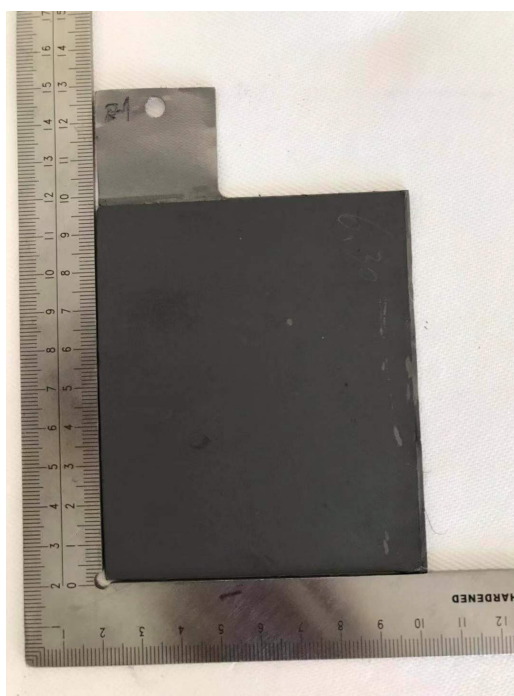
Figure S24. 80 cm 2 cathode sheet used in 5, 65 and 200 Ah industrial-level LMO|AGM+CH@AGM|Zn cells. Photo credit: Shengkai Li, University of Waterloo.
