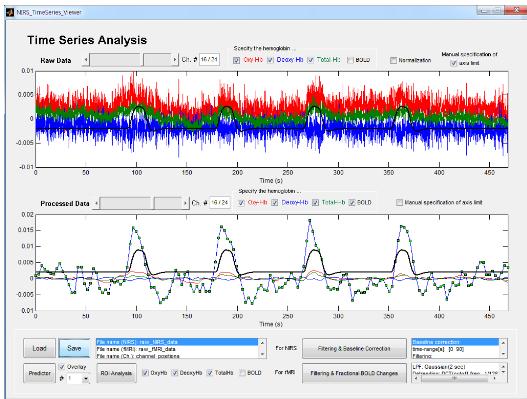
Fig. 14. The window for ‘Time Series Analysis’ routine. The upper figure is the time series of \Delta\text{HbO} , \Delta\text{HbR} , \Delta\text{HbT} , and BOLD data without filtering. Another figure is the time series of filtered \Delta\text{HbO} , \Delta\text{HbR} , \Delta\text{HbT} (Gaussian smoothing, FWHM 2 sec, wavelet-MDL detrending), and BOLD relative to its baseline (Gaussian smoothing, FWHM 2 sec, DCT-based detrending, cut-off: 128 sec). Red line is \Delta\text{HbO} , blue line is \Delta\text{HbR} , green line is \Delta\text{HbT} , blue line with green marker is BOLD, and black line is a predicted model.
