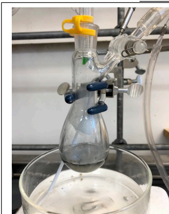
Image 4. Reaction after addition of the catalyst solution via syringe under N 2 .
