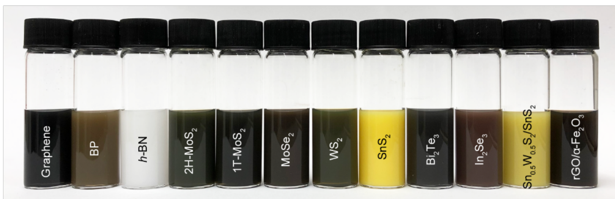
Fig. S5. Photograph of the formulated inks in this work. This includes graphene, BP, TMDs (2H-MoS 2 , MoSe 2 , WS 2 ) and Bi 2 Te 3 produced via LPE, h -BN, 1T-MoS 2 and In 2 Se 3 produced via ion intercalation, SnS 2 and Sn 0.5 W 0.5 S 2 /SnS 2 produced via chemical synthesis, and rGO/ \alpha -Fe 2 O 3 produced via hydrothermal synthesis. Typical ink concentration is \sim 1 \text{ gL}^{-1} . Photo Credit: Guohua Hu, University of Cambridge and The Chinese University of Hong Kong.
