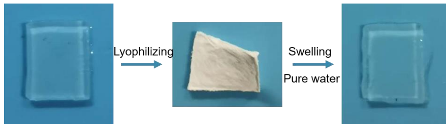
Supplementary Figure 18. Photos of the hydrogel swollen in pure water (left), after drying (middle) and reswelling (right).
