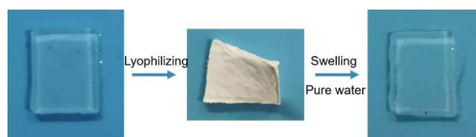
Fig. S18. Photos of the hydrogel swollen in pure water (left), after drying (middle) and reswelling (right). (On page 10 of SI)
