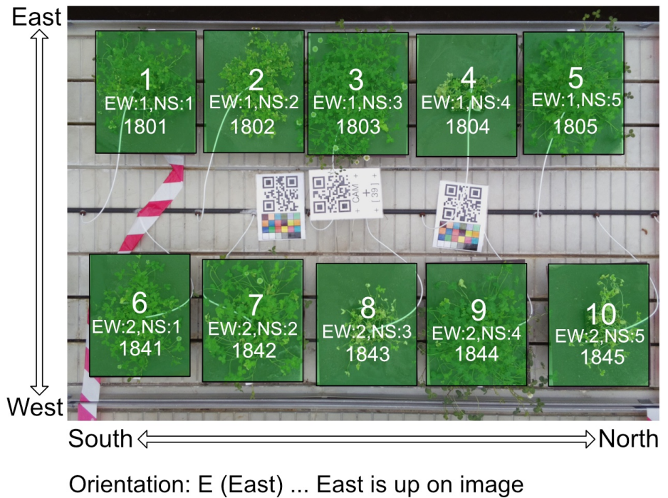
Figure S7. Demonstration of the Pot identification. Name map and Camera map formatted in the CSV (Comma Separated Values) format. Name map contains NS and EW coordinates for each individual pot encoded as a Barcode. Camera map contains the Cam ID and the range of NS and EW coordinates covered by the camera, and in which orientation the camera is placed in the NS and EW space. The example image is represented as Camera 1 (physical camera ID) known from the image filename. The orientation is E (East) since east is up on the image. The numbers on each green block represent the order in which the coordinates are given. The EW:n,NS:n describe the given coordinate to the pot and number below is the corresponding barcode given to the pot.
