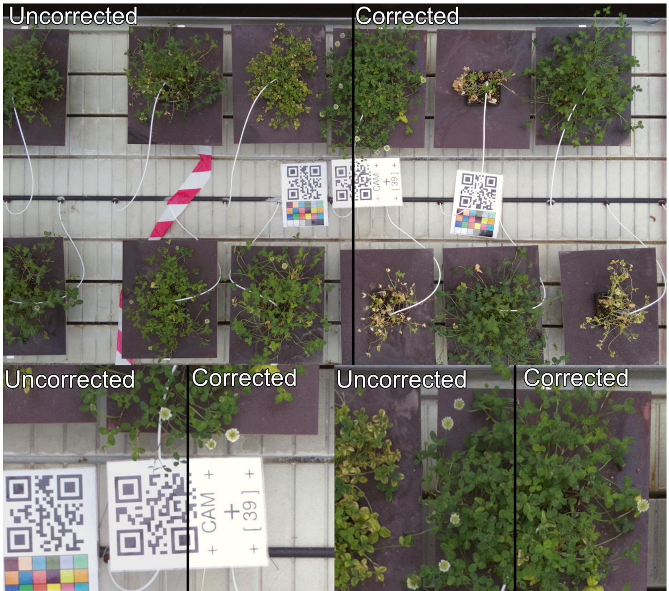
Figure S8. Color correction demonstration using white balance correction based on the QR code white color. Left side is uncorrected having a darker tint and the right side is corrected into being slightly brighter. Below are zoomed in parts of the QR code and the plant above it.
