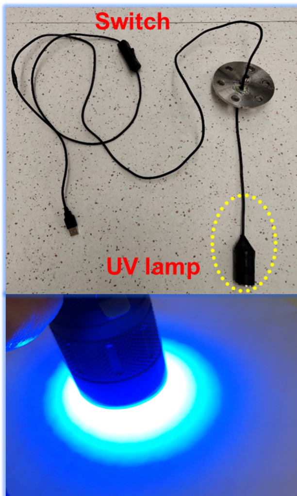
Fig. S10. Permeation cell equipped with UV lamp. Photo credits: Jiangtao Liu.
