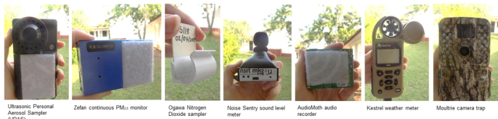
Figure 3. Images of environmental monitoring equipment.
