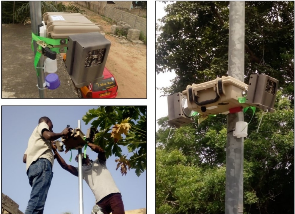
Figure 5. Deployment of the pollution measurement equipment.
