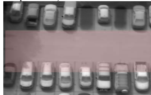
Surface temperature simulated (street and pavement): 47.0-54.4 °C
