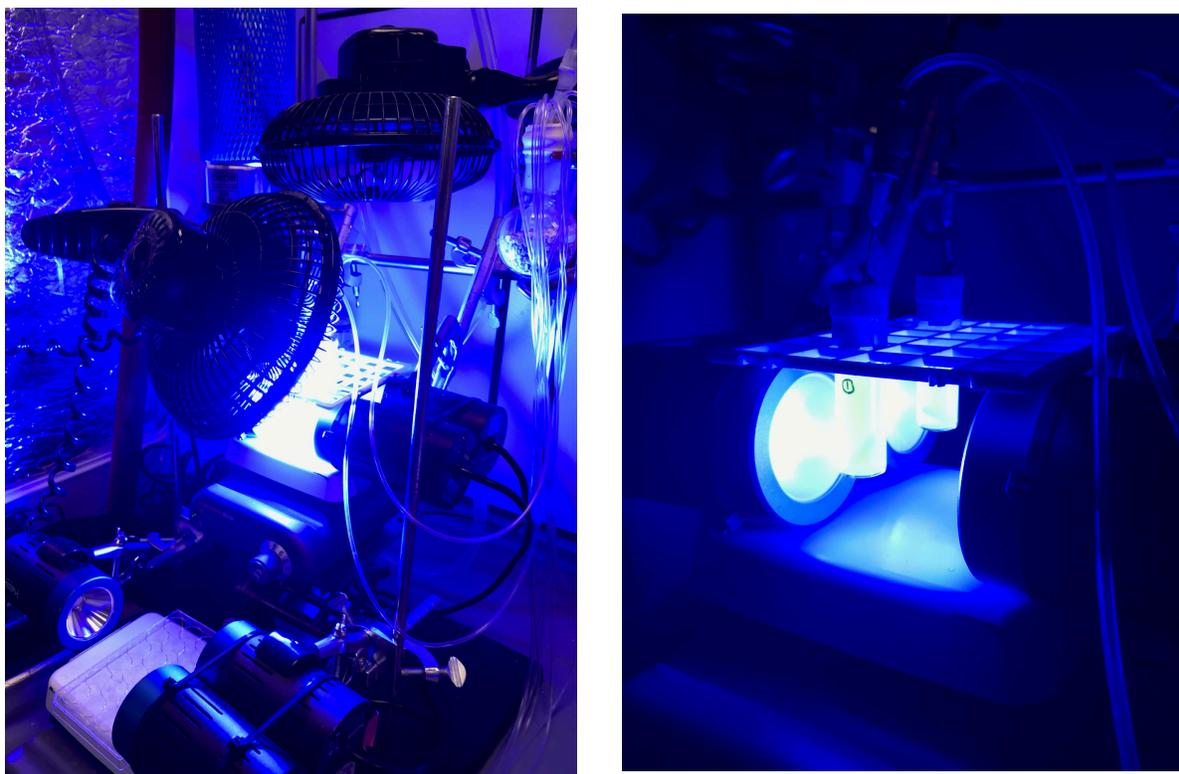
**Figure S2.** Set-up for preparative scale hydroetherification reactions under blue light irradiation.
