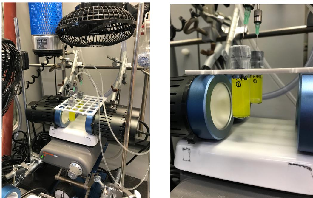
**Figure S1.** Set-up for preparative scale hydroetherification reactions.
