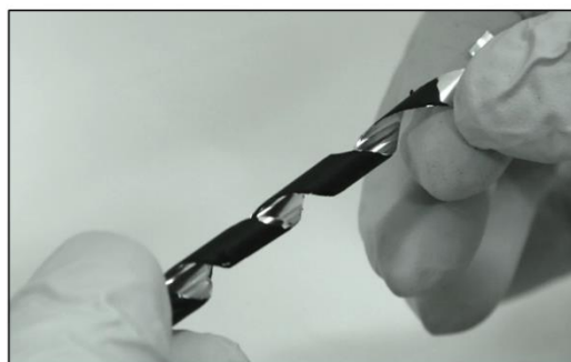
Figure S1. Roll-to-roll coated TIPS LFP electrode on Al current collector under various mechanical deformation. TIPS electrode did not show any sign of delamination confirming the manufacturability in relevant industrial processes.
