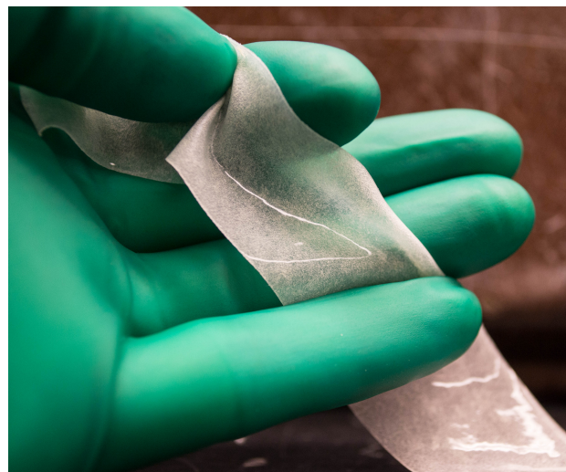
Supplemental Figure 1. Integra Dermal Regeneration Template. The scaffold comprises of two layers, an outer layer made of a thin silicone film that acts as an epidermis and an inner layer constructed of a complex matrix of cross-linked fibers that enables re-growth of the dermis.
