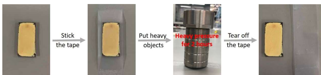
Supplementary Figure 41. Adhesion test of the CN TM film on FTO by tape bonding. After ultrasonication, the CN TM electrode underwent the shown process of tape bonding.
