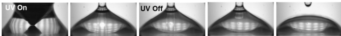
Figure R14. Optical captures the one-droplet 3D printing process when the volume of the droplet is bigger than the volume of the intended structure.
