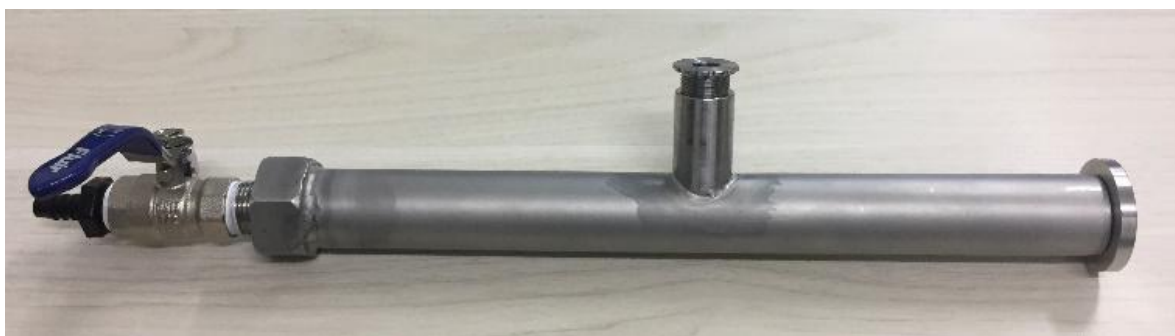
Figure S1. Hand-made reactor for functionalization of ETT with curcumin.
