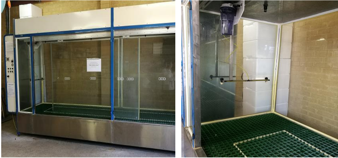
FIGURE S1 The cabinet spray chamber (TeeJet XR11001 flat fan, Spraying Systems Co, Wheaton, IL, USA) used for metribuzin spray.
