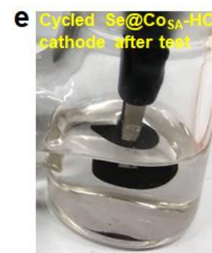
Supplementary Figure 36. Visual observation of lithium polyselenide dissolution in the electrolyte before and after cycling (3 cycles) using two types of cycled cathodes for a comparison. (a) H-type cell for Li–Se batteries, (b) cycled bare Se@HC cathode before test, (c) cycled bare Se@HC cathode after test, (d) cycled Se@Co SA -HC cathode (after 1700 cycles) before test, (e) cycled Se@Co SA -HC cathode after test.
