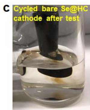
Supplementary Figure 36. Visual observation of lithium polyselenide dissolution in the electrolyte before and after cycling (3 cycles) using two types of cycled cathodes for a comparison. (a) H-type cell for Li–Se batteries, (b) cycled bare Se@HC cathode before test, (c) cycled bare Se@HC cathode after test, (d) cycled Se@Co SA -HC cathode (after 1700 cycles) before test, (e) cycled Se@Co SA -HC cathode after test.
