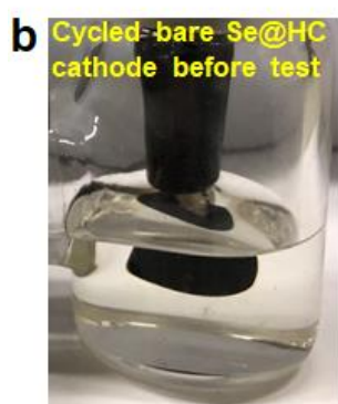
Supplementary Figure 36. Visual observation of lithium polyselenide dissolution in the electrolyte before and after cycling (3 cycles) using two types of cycled cathodes for a comparison. (a) H-type cell for Li–Se batteries, (b) cycled bare Se@HC cathode before test, (c) cycled bare Se@HC cathode after test, (d) cycled Se@Co SA -HC cathode (after 1700 cycles) before test, (e) cycled Se@Co SA -HC cathode after test.
