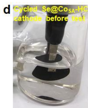
Supplementary Figure 36. Visual observation of lithium polyselenide dissolution in the electrolyte before and after cycling (3 cycles) using two types of cycled cathodes for a comparison. (a) H-type cell for Li–Se batteries, (b) cycled bare Se@HC cathode before test, (c) cycled bare Se@HC cathode after test, (d) cycled Se@Co SA -HC cathode (after 1700 cycles) before test, (e) cycled Se@Co SA -HC cathode after test.
