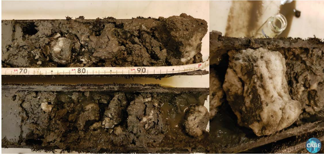
Supplementary figure 3: Pictures of gas hydrate nodules retrieved within 0.7-1.2 mbsf on gravity core CAGE17-5_1401 (Cruise report - https://cage.uit.no/cruise/geomorphic-mapping-seismic-stratigraphy-cruise/ ). Photo/Image courtesy of Karin Andreassen (CAGE-UiT The Arctic University of Norway).
