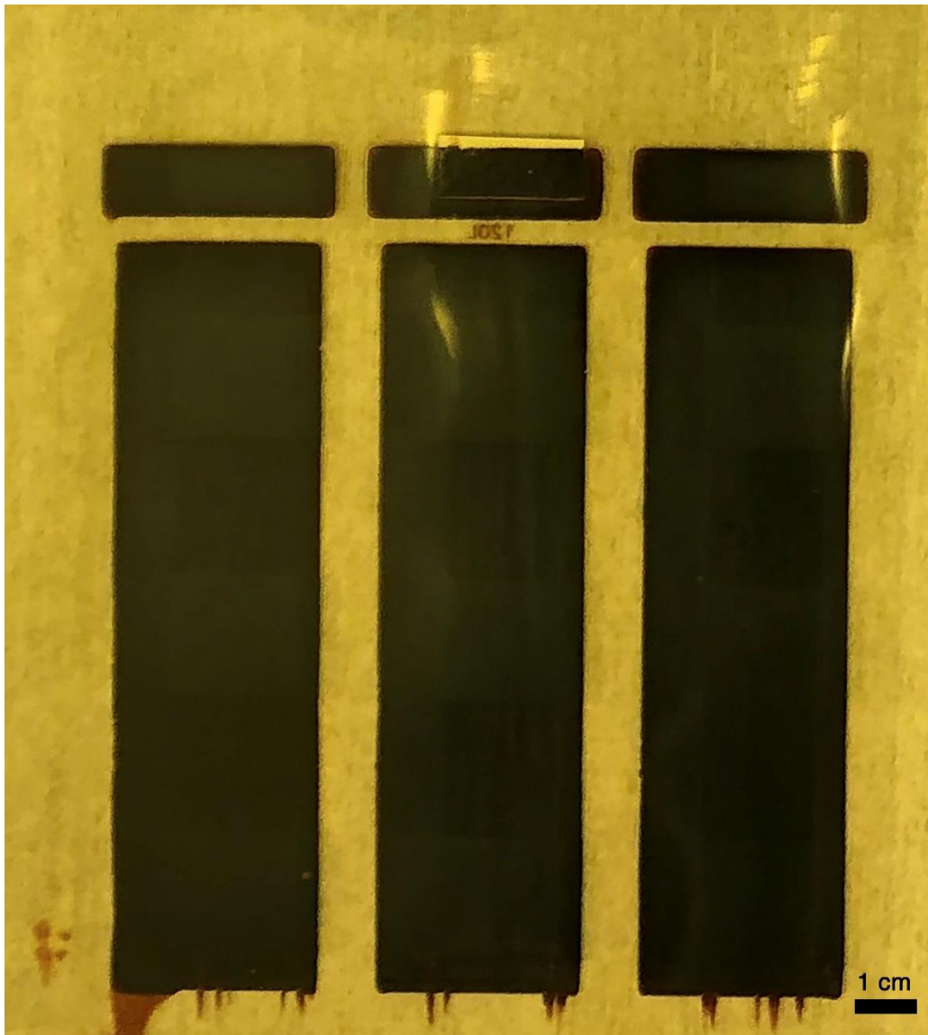
Supplementary Figure 12. A picture of A4-paper-sized film of gravure-printed perovskite on the PET/ITO/SnO 2 .
