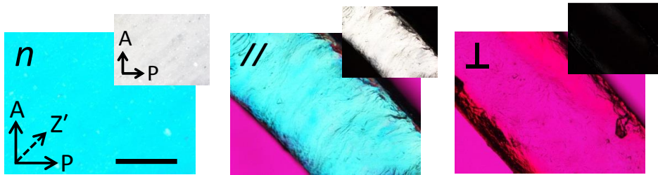
Supplementary Fig. 7. Anisotropic structure of the monodomain hydrogel in the as-prepared state. POM images of the as-prepared hydrogel viewed from different directions. Scale bar, 1 mm.
