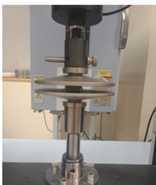
Figure S1. Compression plates set-up used for static compression test.
