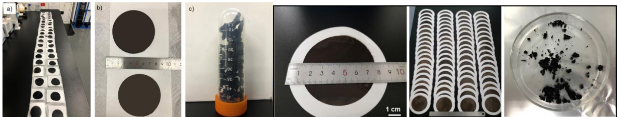
Figure A: Pictures of a number of CNT-EP-PC15 membranes prepared for the gas adsorption studies.
