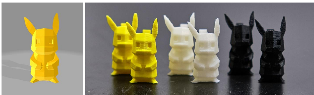
Figure S1. A 3D model of a low-poly Pikachu ( thingiverse.com/thing:376601 , left) and figurines printed out of yellow, natural and black ABS filament (right).
