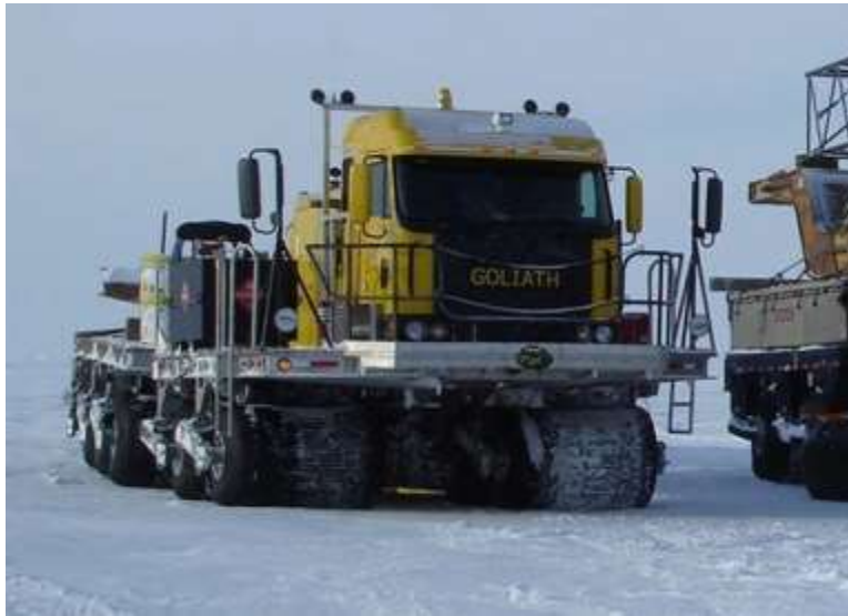
Figure S8. Rolligons - vehicles with large, low-pressure tires used by the oil industry in Canada and Alaska. The SAExploration plan of operations listed one Rolligon per crew (SAExploration 2018). (Photo: Alaska Department of Natural Resources)
