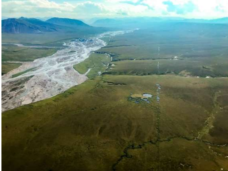
Figure S21. One of many bladed tractor trails just west of the Canning River and the Arctic National Wildlife Refuge, caused by seismic exploration in the 1960s, photographed in 2018. Note the extensive thermokarst and ponding of water along the trail and around the gravel drilling pad near the center of the photo, abandoned since 1974. (Photo: M. Nolan, Fairbanks Fodar, http://fairbanksfodar.com/happy-10-02-day . Accessed 28 July 2018)
