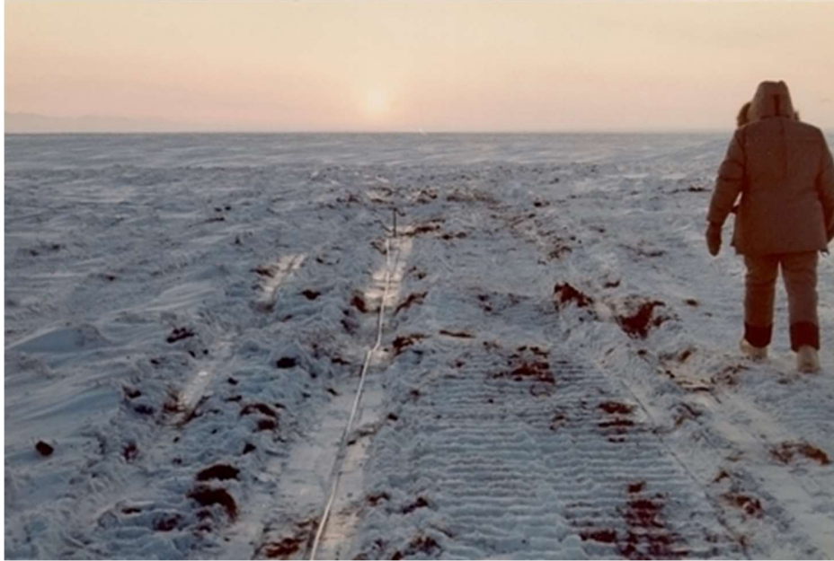
Figure S12. Trail made by Caterpillar D7 tractors and ski-mounted trailers in March 1984 in the 1002 Area of the Arctic National Wildlife Refuge. This site was still highly disturbed in 1994 (Jorgenson et al. 1996). By 2018 the trail here had subsided into a large pond due to melting of ice wedges (Jorgenson 2018). Based on the amount of exposed soil in the tracks, it is clear that there was insufficient snow to protect the tundra. (Photo: U.S. Fish & Wildlife Service)
