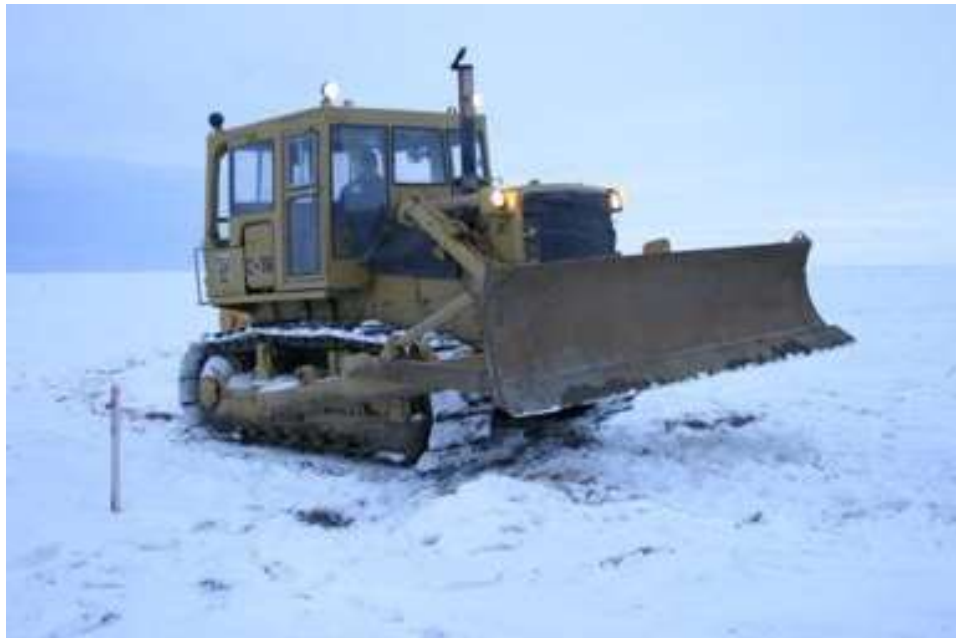
Figure S7. Caterpillar D7 steel-tracked dozer used to haul heavier Cat-train camps and equipment. The SAExploration plan of operations included two of these per crew (SAExploration 2018). However four were used per crew at GMT 3-D in 2017 in an area that was flatter than the 1002 Area. (Photo: Alaska Department of Natural Resources)
