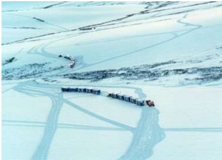
Figure S5. Five Cat-trains with sled-mounted trailers during 3D seismic exploration in hilly terrain near Kavik, west of the 1002 Area, 2001. The three Cat-trains in background apparently required two tractors per train to travel in this hilly terrain (one D7 to assist the lighter tractor), while the two trains in the foreground were waiting for tractors to return for them. (Photo: U.S. Fish & Wildlife Service)
