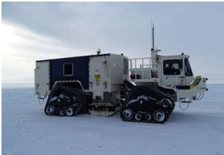
Figure S2. The rubber-tracked Inova AHV-IV Vibroseis vehicle. The vibrator pad is located between the front and rear treads of the vehicle. The SAExploration plan of operations included 12 of these per crew (SAExploration 2018). (Photo: Bureau of Land Management)
