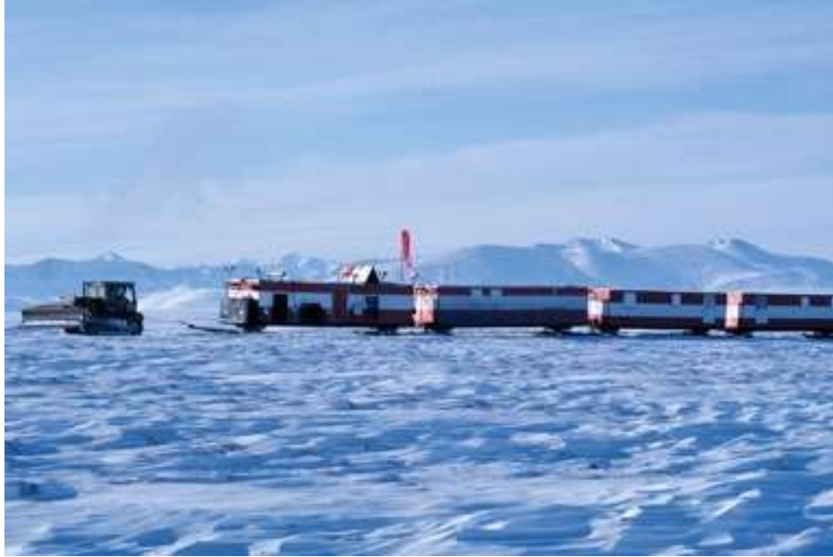
Figure S4. Cat-train of sled-mounted camp trailers pulled by a Caterpillar D7 dozer during the 1984–1985 surveys in the 1002 Area of the Arctic National Wildlife Refuge. The SAExploration plan of operations proposed one 150-person camp per crew (SAExploration 2018). The vehicles required for the mobile camps consist of 8–10 strings of 5–8 sleds pulled by large tractors. (Photo: U.S. Fish & Wildlife Service)
