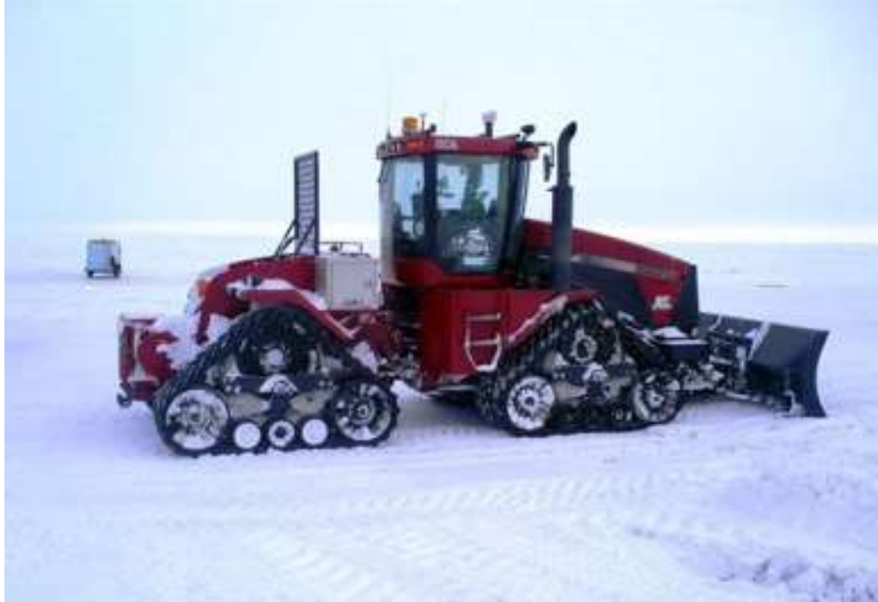
Figure S6. Steiger tractor used to haul camp trailers and other vehicles and equipment. The SAExploration plan of operations anticipated nine Case/Steiger tractors per crew (SAExploration 2018). (Photo: Alaska Department of Natural Resources)
