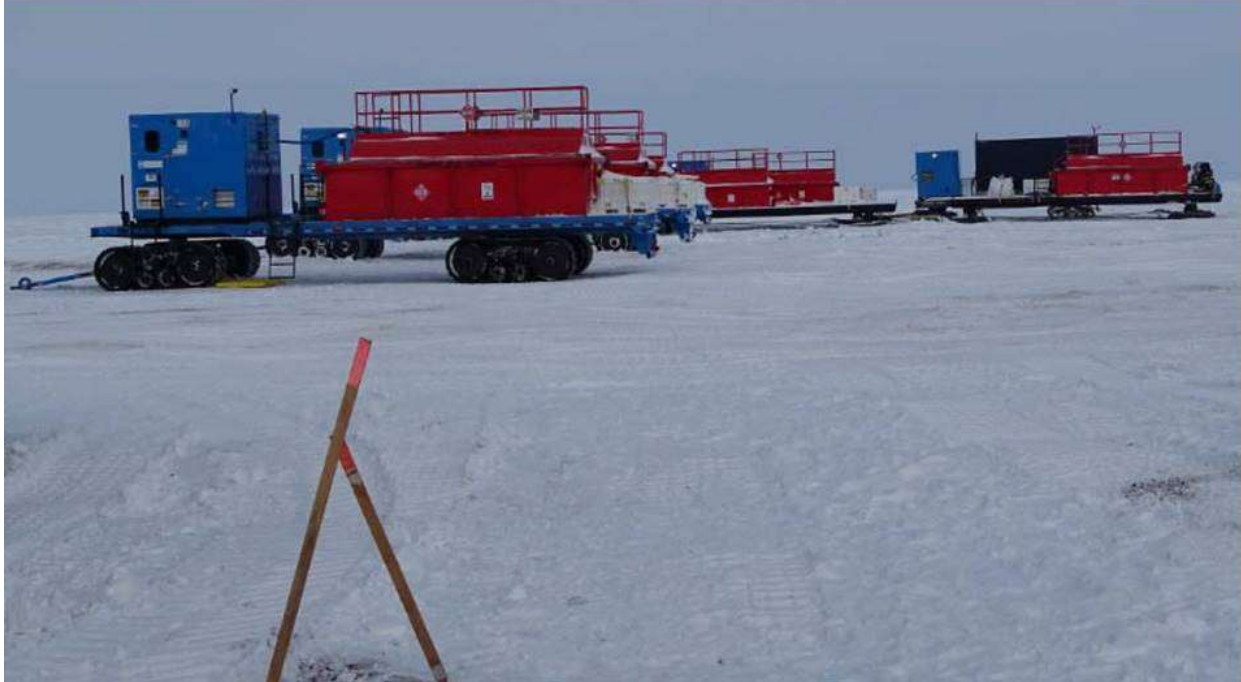
Figure S10. Fuel tanks on trailers. These trailers would be used to deliver 6,000 – 7,000 gallons of fuel every day to the camps in the 1002 Area (SAExploration 2018). (Photo: Bureau of Land Management)
