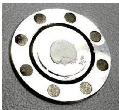
Figure S4. Example of target that was left exposed to the elements for too long, resulting in the CaO target material absorbing moisture and resulting in rupture. The target could not be used for irradiation.
