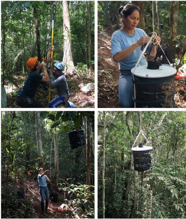
Fig S1. BG-Sentinel trap placement in a tree using BigShot slingshot. Top L-R: lead weight and fishing line being launched over a branch to which a rope is attached; trap being prepared. Bottom L-R: trap being raised to desired height; trap hanging at 10 m from a tree.
