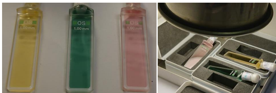
Figure S5. Photograph of [\text{Fe}(\text{phtmeimb})_2](\text{PF}_6)_2 , [\text{Fe}(\text{phtmeimb})_2](\text{PF}_6) and [\text{Ru}(\text{bpy})_3](\text{PF}_6)_2 under illumination. Left) From left to right: [\text{Ru}(\text{bpy})_3](\text{PF}_6)_2 (yellow), [\text{Fe}(\text{phtmeimb})_2](\text{PF}_6)_2 (green) and [\text{Fe}(\text{phtmeimb})_2](\text{PF}_6) (light red) in acetonitrile. Right) Samples under compact fluorescent lamp for stability test.
