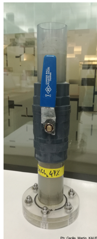
Fig. S4 Sediment-Microplastic Isolation (SMI) unit (design and picture) adapted from the design proposed by Coppock et al., 2017. Differences from the original design include use of poly methyl methacrylate (PMMA) instead than polyvinyl chloride (PVC) tubes and removable base to ease washing. Photo credit: Cecilia Martin, King Abdullah University of Science and Technology.
