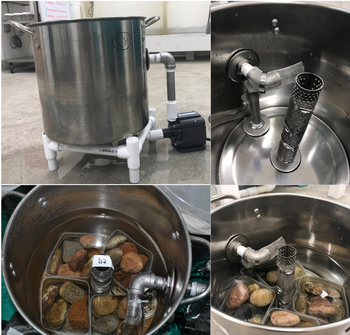
Figure S1. Example of an experimental stream. Each stream mesocosm is constructed from a 15.1-L stainless-steel pot, outfitted with a magnetic-drive pump (Danner Supreme® model 3). The stream contains a 12.7-cm stainless-steel drainpipe covered with 1-mm metal mesh and a 21-cm perforated stainless-steel recirculation pipe surrounded with 1-mm wire mesh. The pump is connected on one end to recirculation pipe and on the other end to a stainless-steel elbow joint located above the water level to provide water flow and create an aerated ripple environment. Each stream contains four rock trays colonized with natural communities. Photo credit: Janet Miller, U.S. Geological Survey.
