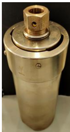
Figure S7. Berghof DAB3 Teflon lined stainless steel high pressure reactor.
