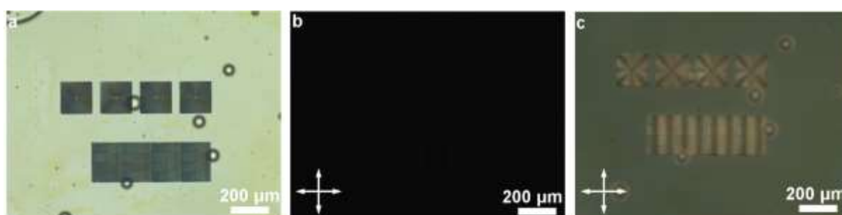
Figure S6. Grating effect from micro-channels. (a) Bright field image of sinusoidal patterns and +2 topological defect patterns. (b) POM image of sinusoidal patterns and +2 topological defect patterns. (c) 100 times exposure of POM image in (b). Note that (a) and (b) have same exposure with images in Figure 1.
