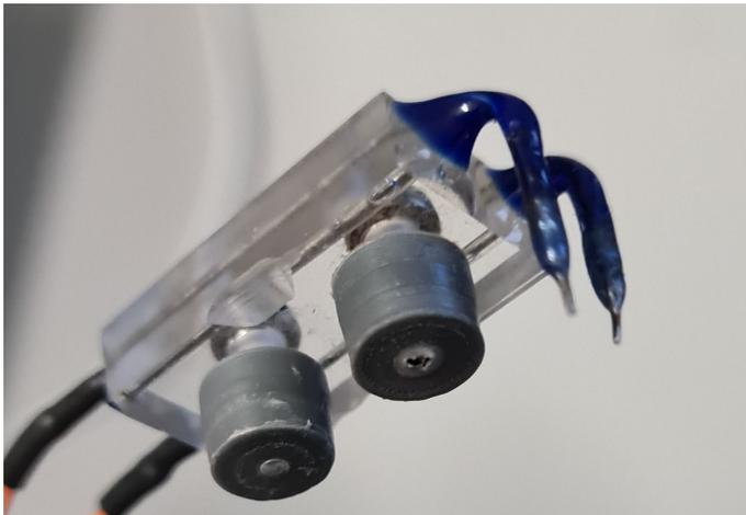
**Supplementary Figure 3: Equipment used for electrical pacing of cardiac MTs. (a) Pulse stimulator connected to custom-made electrodes fitting the V-shaped 96-wells and (b) details of custom-made electrodes.**
