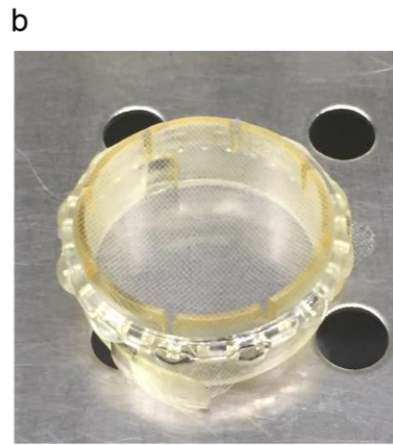
Supplementary Figure 3. Scaffold preparation for cell culture. a) Schematic of cell crown and scaffold assembly. b) Photograph of a PCL scaffold fabricated by MEW and assembled in cell crown holder.
