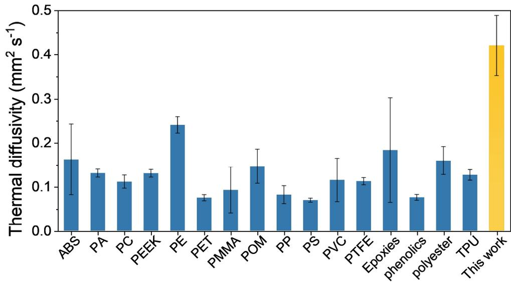
**Supplementary Figure 7 | Comparison of thermal diffusivity.** Comparison of thermal diffusivity of the all-natural bioinspired structural material with typical polymers<sup>1</sup>.
