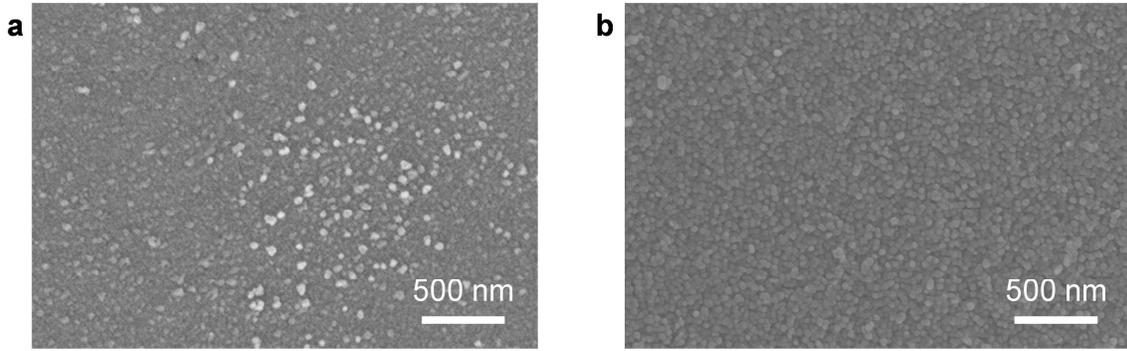
**Supplementary Figure 3 | The comparison of the unique connected-nanograin structure between natural nacre and the all-natural bioinspired structural material. a, Surface of *Anodonta woodiana*. b, Surface of the all-natural bioinspired structural material.**
