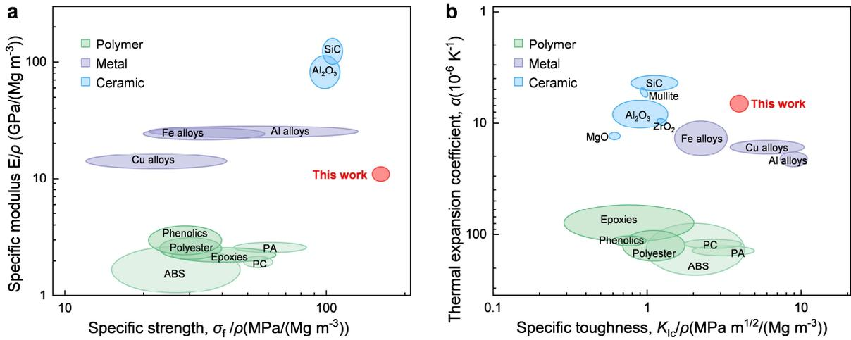
**Supplementary Figure 8 | Comparison of thermal and mechanical properties of all-natural bioinspired structural material with typical polymers, metals, and ceramics. a, Ashby diagram of specific modulus versus specific yield strength<sup>1,2</sup>. b, Ashby diagram of thermal expansion versus specific fracture toughness<sup>1,2</sup>.**
