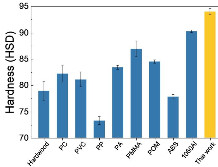
**Supplementary Figure 9 | Comparison of hardness.** Comparison of Shore D hardness number of the all-natural bioinspired structural material with other widely used materials. Error bars represent standard deviation.
