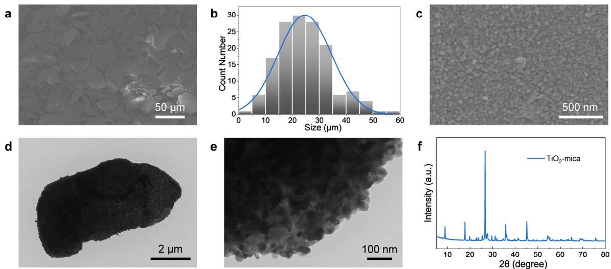
**Supplementary Figure 2 | Characterization of TiO<sub>2</sub> coated mica microplatelet (TiO<sub>2</sub>-mica).**
