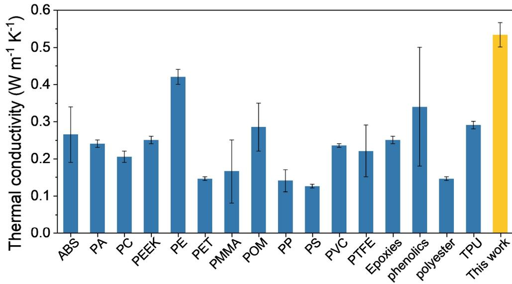
**Supplementary Figure 6 | Comparison of thermal conductivity.** Comparison of thermal conductivity of the all-natural bioinspired structural material with typical polymers<sup>1</sup>.
