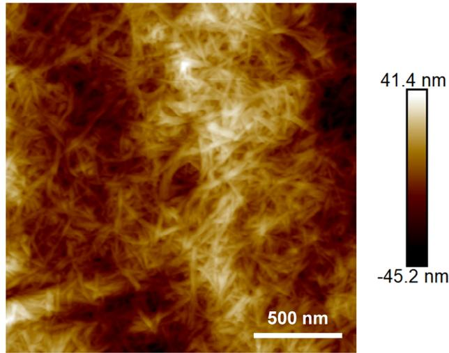
**Supplementary Figure 1 | Atomic force microscope (AFM) image of TEMPO-oxidized cellulose nanofiber (CNF).**
