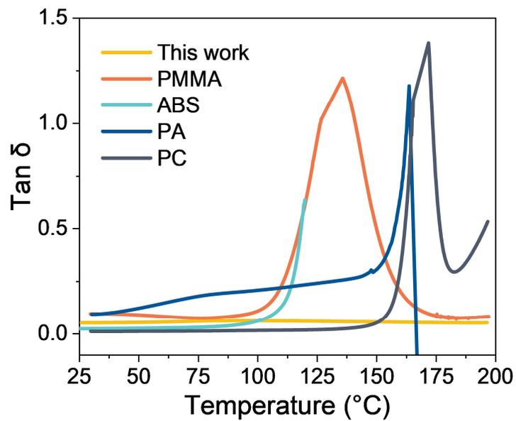
**Supplementary Figure 5 | Comparison of loss factor ( $\tan \delta$ ).** The curves show that  $\tan \delta$  of the all-natural bioinspired structural material is more stable than widely used petroleum-based plastics under temperature ranging from 30 °C to 190 °C.
