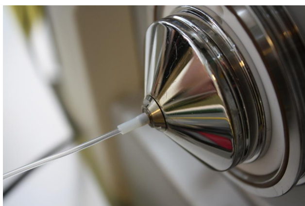
Figure S-3. The flexible ion transfer tubing of the DESI/EASI/LTP source was directly connected to the heated capillary of a LTQ-Orbitrap XL mass spectrometer (Thermo Fisher Scientific GmbH) using a PTFE sleeve.
