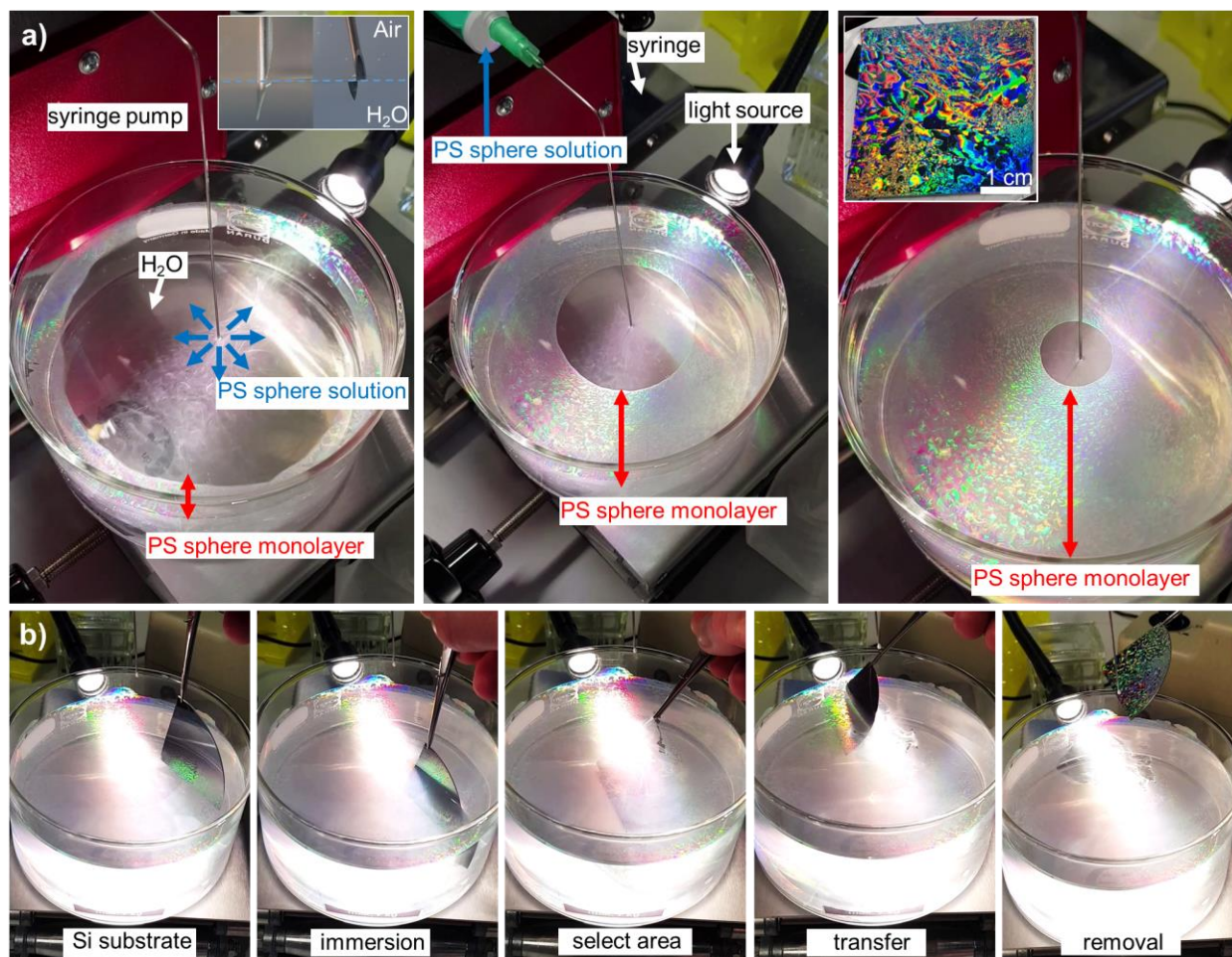
Figure S 1. Self-Assembly of a PS sphere monolayer ( d = 1100 nm) on the water-air interface and transfer to a Si substrate.
