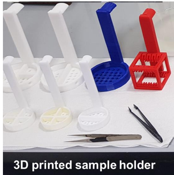
Figure S 4. HF resistant 3D printed sample holders (polylactic acid, PLA).
