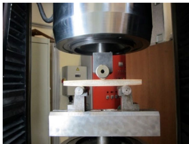
Figure S2: The three-point bending test performance using the servo-hydraulic testing machine INSTRON 1255.
