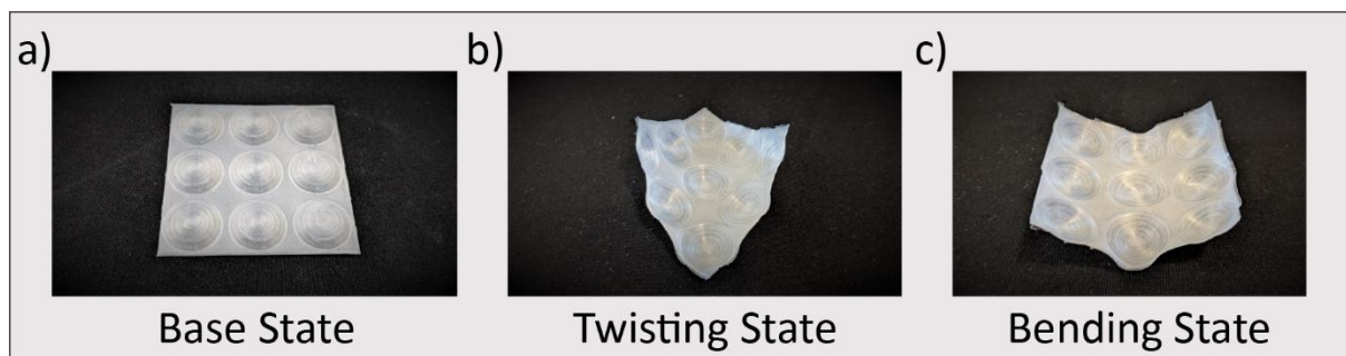
Figure S10: 3D printed Nylon sheet displaying a square array of 3 \times 3 square domes in the (a) as-printed base state (no domes inverted), (b) twisting state with all domes inverted and, (c) bending state with the domes inverted.
