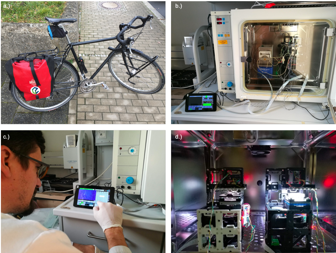
Figure 14. Setting up the incubator-enclosed microscope - a) The microscope fits inside a small box and can conveniently be printed and assembled and transported to the bio-lab using a commuter bag on a bike. In b) we show a customized application, where a microfluidic Ibidi \mu -chip with endothelial/macrophage perfused co-culture was placed on the incubator-enclosed microscope, before all cables were connected. c) The next step requires setting up experimental details such as duration and interval, as well as illumination settings using the touch-screen on the GUI. d) due to their small footprint multiple devices fit inside a single incubator for multiplexed experiments.
