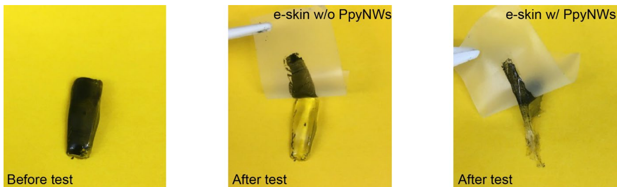
Fig. S13. Photographs showing the different surface adhesion of MXene and MXene-PpyNW composites to VSNP-PAM hydrogels with 3M tape peeling tests. (Photo credit: Yichen Cai, and Jie Shen, KAUST)
