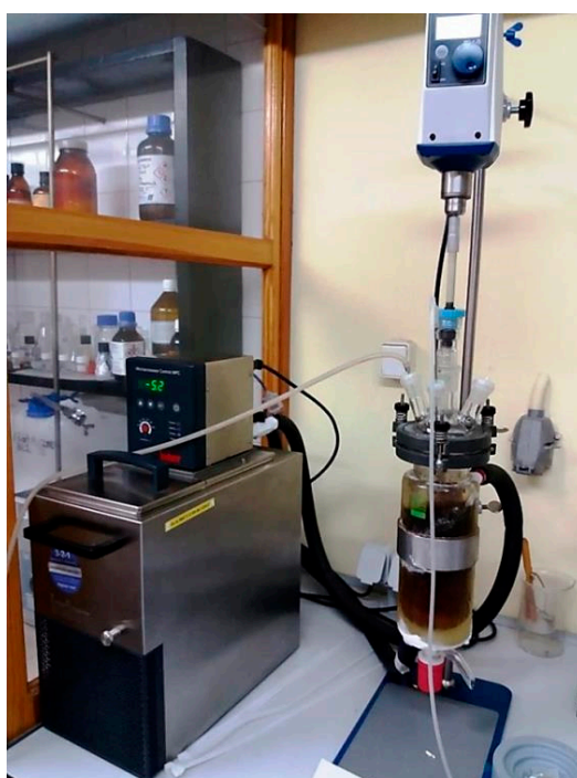
Figure S1. The photograph of the lab set employed for the N-AgNPs preparation taken during the synthesis.
