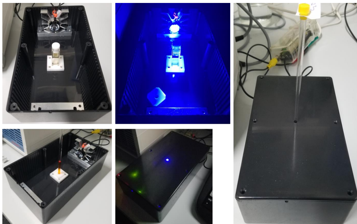
Figure S1: In-house built LED irradiation box for UV/Vis cuvettes as well as NMR tubes.
