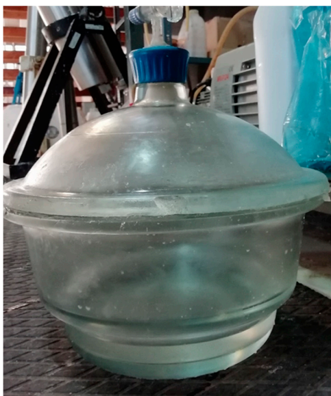
Figure S1. Desiccator used for vacuum saturation of the core plugs.
